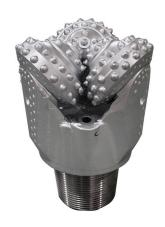
On the left is a tri-cone drill bit, on the right is a percussive drill bit. Getting the exact diameter is not easy.
